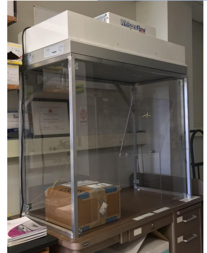
Fig 2: Clean Room Hood and Air Filter
